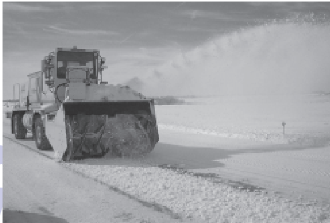
Blowers can throw snow 150' at a rate of 6,000 tons/hour. Operations can keep pace with a snowfall at a rate of one inch/hour.
