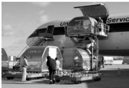
K-Lift Loader puts packages into jet. During peak, farm tractors are used for tugs to push planes out.
